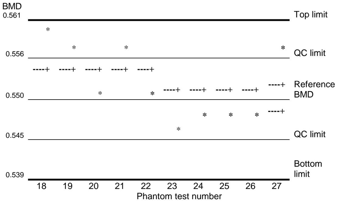
NOTE: Phantom BMD (\*) must be within top/bottom limits.
