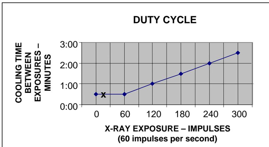
The accuDEXA pulses last approximately 0.14 seconds, which is equivalent to 8.4 pulses (indicated by the x in the above graph).
