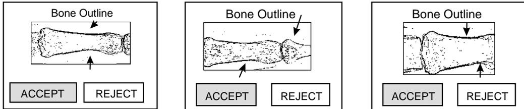
The following images are unacceptable. The image on the left is unacceptable because the sensor did not completely capture both sides of the middle finger (as shown by the arrow). The image on the right is unacceptable because a ring is within the field of view. These images will yield inaccurate results and should be rejected.
