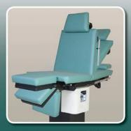
Power adjustment of height (24"–40"), back (flat – 80°), tilt (flat – 30°) and foot sections (vertical – horizontal) allows table to be positioned for various exams and procedures including chair, contoured chair, Trendelenburg, Lithomy, OBGYN and flat.
